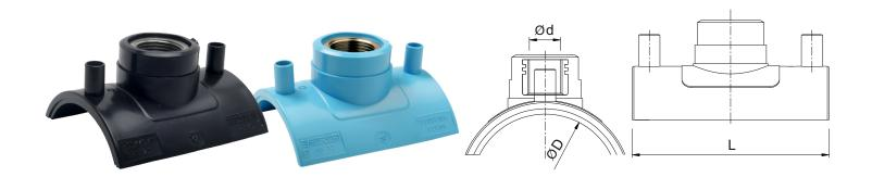
Kimplas Electrofusion Flexi-Fit Branch Tapping Saddles are manufactured in PE 80 (Black) material with threaded metal insert outlets and are of SDR 11 rating (PN 12.5). For exact recommendations on compatibility, for welding with SDR 9 through SDR 21 or PN 6 through PN 16 pipe, refer Kimplas Technical Specifications Manual. Kimplas Electrofusion fittings are suitable for permanently connecting drinking water distribution MDPE 80 and PE 100 pipes, both in straight form as well as in coil form.
