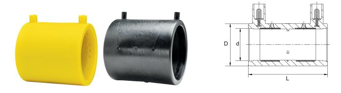
kimplas electrofusion couplers are manufactured in PE 80 (Yellow) & PE 100 (Black) material and are of SDR 11 rated. Kimplas Electrofusion fitings are suitable for permanently connecting to PE 80 and PE 100 pipes, both in straight as well as in coil form.
