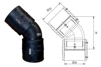
Kimplas Electrofusion Elbows Higher Size are manufactured in PE 100 (Black) material and are of SDR 11 rating (PN 16) rated. For exact recommendations on compatibility, for welding with SDR 9 through SDR 21 or PN 6 through PN 16 pipe, refer Kimplas Technical Specifications Manual. Kimplas Electrofusion Elbows are suitable for permanently connecting MDPE 80 and PE 100 pipes, both in straight as well as in coil form.
