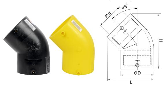
Kimplas Electrofusion Elbows are manufactured in PE 80 (Yellow) and PE 100 Black material and are of SDR 11 rating (PN 16). For exact recommendations on compatibility, for welding with SDR 9 through SDR 21 or PN 6 through PN 16 pipe, refer Kimplas Technical Specifications Manual.Kimplas Electrofusion Elbows are suitable for permanently connecting MDPE 80 and PE 100 pipes, both in straight as well as in coil form.
