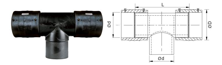
Kimplas Electrofusion Equal Tee are manufactured in PE 100 (Black) material and are of SDR 11 rating (PN 16). For exact recommendations on compatibility, for welding with SDR 9 through SDR 21 or PN 6 through PN 16 pipe, refer Kimplas Technical Specifications Manual. Kimplas Electrofusion fittings are suitable for permanently connecting PE80 and PE100 pipes, both in straight as well as in coil form.
