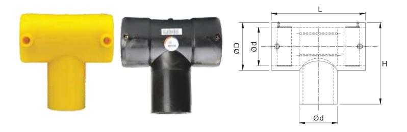
Kimplas Electrofusion Equal Tees are manufactured in PE 80 (Yellow) & PE 100 (Black) material and are of SDR 11 rating. For exact recommendations on compatibility, for welding with SDR 9 through SDR 21 or PN 6 through PN 16 pipe, refer Kimplas Technical Specifications Manual. Kimplas Electrofusion fittings are suitable for permanently connecting to PE 80 and PE 100 pipes, both in straight as well as in coil form.
