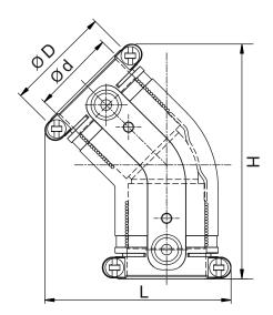
Kimplas Electrofusion 45° Elbows are manufactured in PE 100 Black material and are of SDR 11 rating (PN 16). For exact recommendations on compatibility, for welding with SDR 9 through SDR 21 or PN 6 through PN 16 pipe, refer Kimplas Technical Specifications Manual. Kimplas Electrofusion fittings are suitable for permanently connecting MDPE 80 and PE 100 pipes, both in straight form as well as in coil form.
