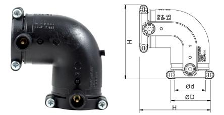
Kimplas Electrofusion 90° Elbows are manufactured in PE 100 Black material and are of SDR 11 rating (PN 16). For exact recommendations on compatibility, for welding with SDR 9 through SDR 21 or PN 6 through PN 16 pipe, refer Kimplas Technical Specifications Manual. Kimplas Electrofusion fittings are suitable for permanently connecting MDPE 80 and PE 100 pipes, both in straight form as well as in coil form.
