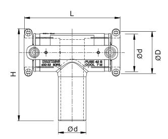
Kimplas Electrofusion Equal tees are manufactured in PE 100 Black material and are of SDR 11 rating (PN 16). For exact recommendations on compatibility, for welding with SDR 9 through SDR 21 or PN 6 through PN 16 pipe, refer Kimplas Technical Specifications Manual. Kimplas Electrofusion fittings are suitable for permanently connecting MDPE 80 and PE 100 pipes, both in straight form as well as in coil form.
