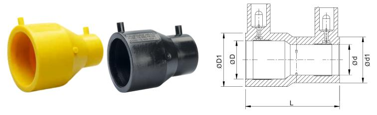
Kimplas Electrofusion Reducers are manufactured in PE 80 (Yellow) and PE 100 Black material and are of SDR 11 rating. For exact recommendations on compatibility for welding with SDR 9 through SDR 21, refer Kimplas Technical Manual. Kimplas Electrofusion Reducers are suitable for permanently connecting PE 80 pipes and PE 100 pipes, both in straight as well as in coil form.
